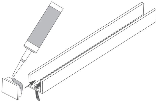
**OPTIONALLY:** Power cables can be run through the end caps in which case the extrusion does not need to be drilled through.
