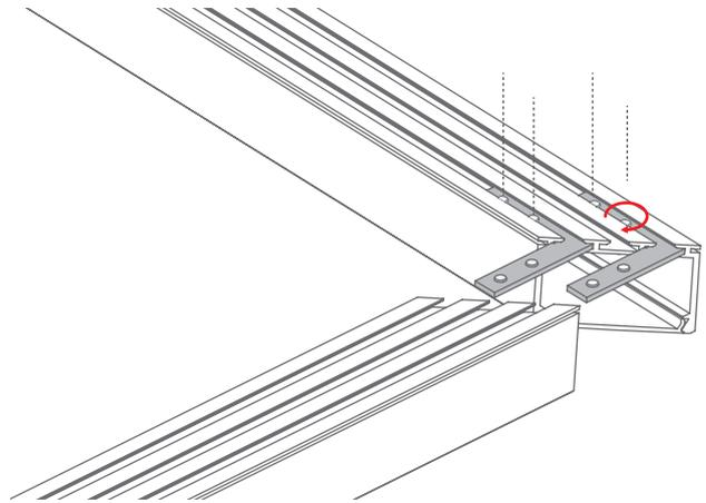
**3.** Slide the other half of the extrusion onto the connectors and tighten the pressure screws with an Allen wrench.
