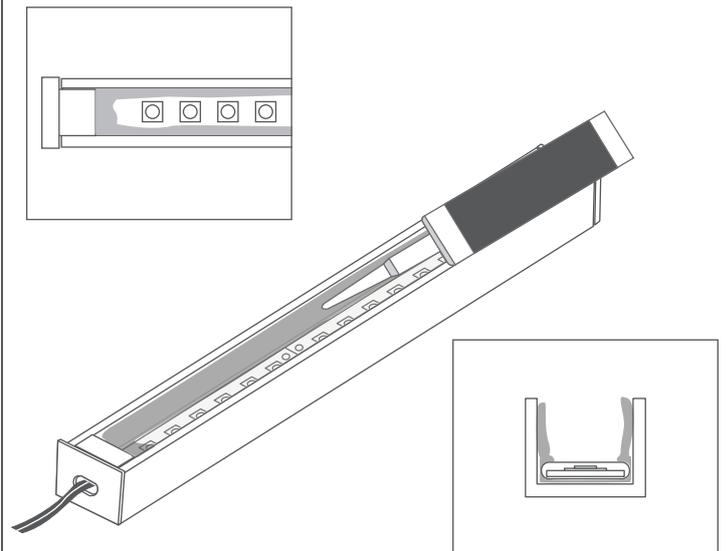
**5.** Remove the excess silicone with a rectangular tool (e.g. a piece of cardboard), taking care not to damage the tape. The silicone layer must be even and must not obscure the LEDs.
