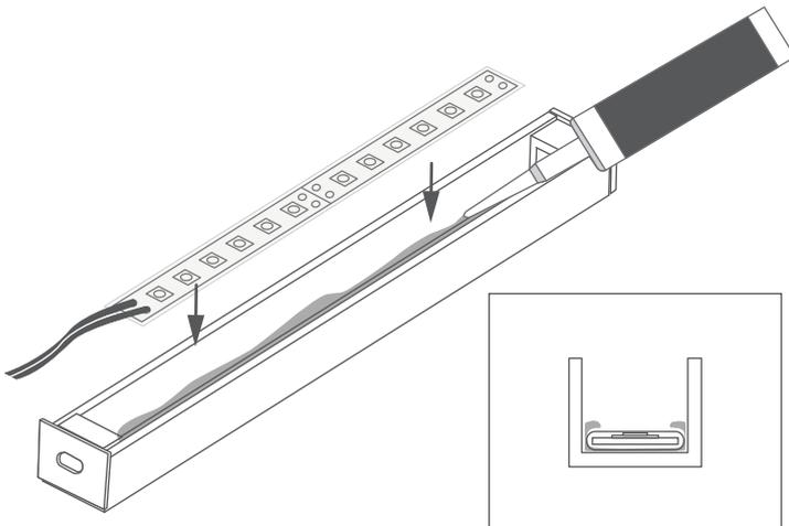
**4.** Apply a second layer of silicone on the extrusion walls and the end caps.
