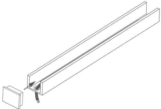
**OPTIONALLY:** The end caps can be attached to the extrusion using glue.
