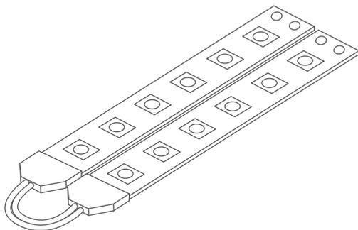
**OPTIONALLY:** The power cords can be led out from one pole of a given strip. This method is used to power suspended lighting fixtures.
