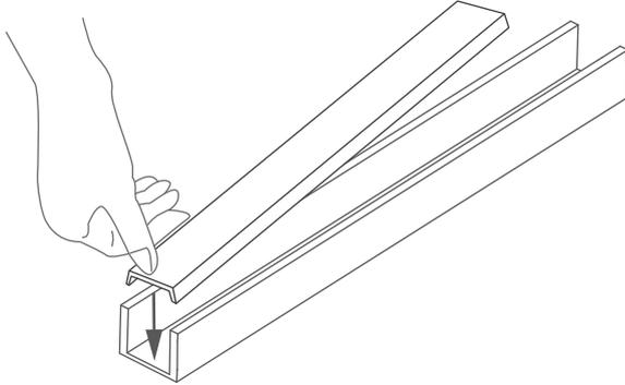
**2.** Press in the subsequent sections of the cover. Be careful not to bend or break the wings of the cover.
