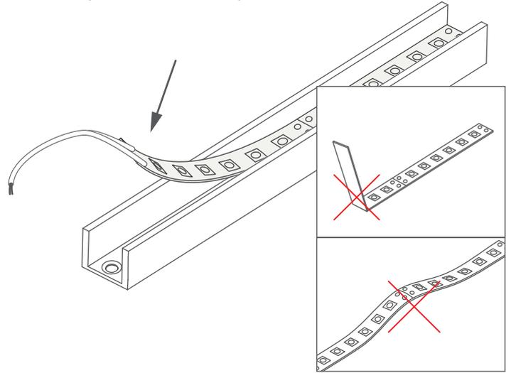
**3.** Lead the power cable through the drilled hole.
