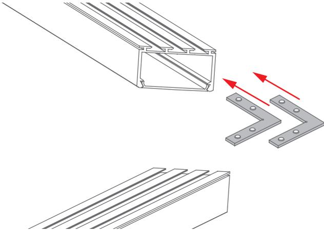
**2.** Tighten the two pressure screws in each connector with an Allen wrench.
