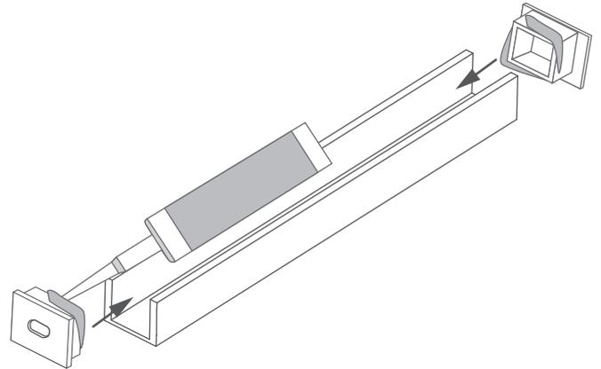
**3.** Apply a silicone layer to the bottom of the profile and embed the LED strip in it.
