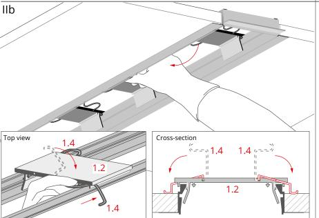
Lock the springs (1.4) at each item (1.2) by turning them, pressing them against the plate surface and sliding under the edge of the item (1.2) as shown in the figure.
