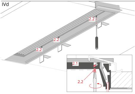
out by tightening the locking bolts (2.2) in the pre-drilled holes.
