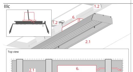
Mount the power supply (6) on the back of the profile in such a position that it fits into the opening of the RAM-KOZE-100 profile.
