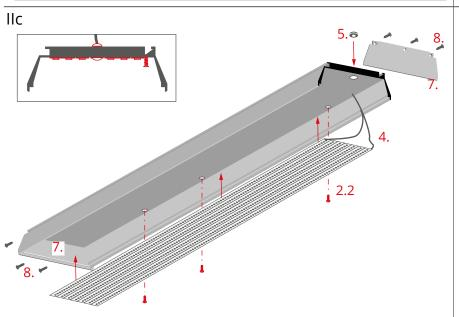
Adhere the LED tapes (4), mount the gland (5) and route the power cable through it.
