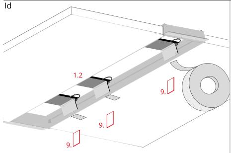
To facilitate further work, mark the location of the items (1.2) in the RAM-KOZE-100 profile, e.g. with colored adhesive tape.
