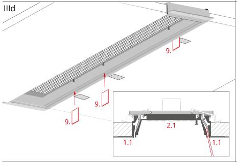
To prevent the OMODO-100 profile from falling out, insert wedges temporarily (9). They should be inserted into the marked spots in the gap between item (1.1) and item (2.1). There should be one wedge for each marked element (1.2) and they should be placed from the side of the profiled orientation line.
