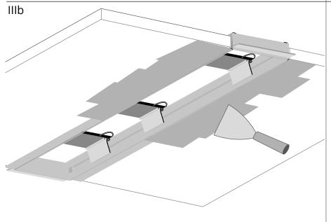
Apply glue and spread it at the junction of the profile's flanges and drywall.
