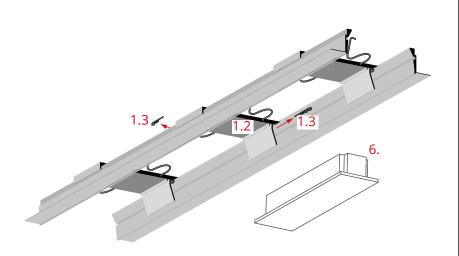
If the power supply (6) does not fit into the openings of the RAM-KOZE-100 profile, its items (1.2) must be slid further apart accordingly.
