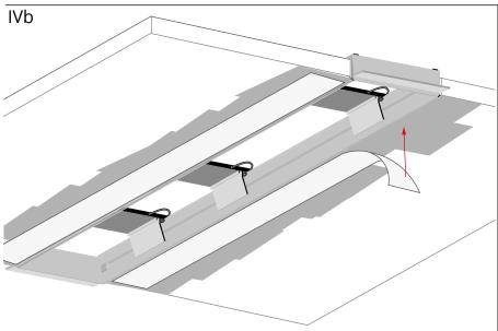
Attach TUFF-TAPE or equivalent at the junction of the profile flanges and drywall.
