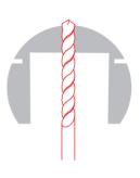
**5.** Bevel the hole so that the plastic screw head fits in.
