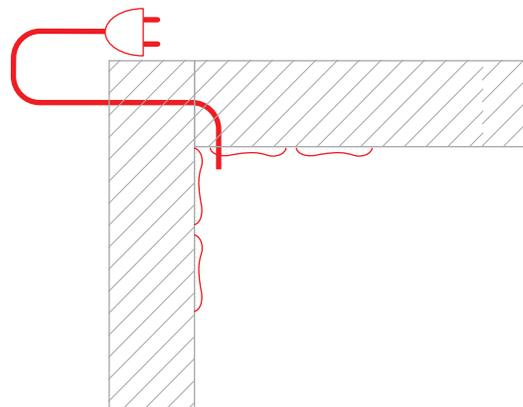
**3.** Connect power to the LED strip and attach the extrusion (A).
