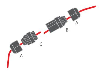
**2.** Connect the cables using e.g. a connection block and place the connection inside the large body (B).
