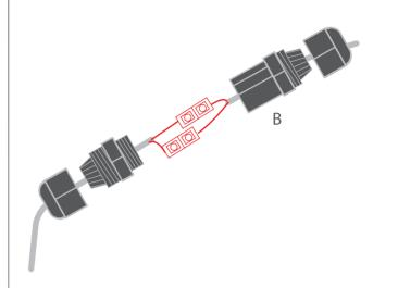
**3.** Connect the small body (C) with the large body (B).
