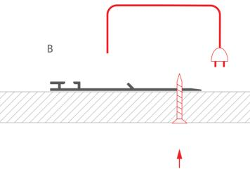
**2.** Feed the power cable. Mount the LED strip (F) insert the cover (C) and end cap (D).
